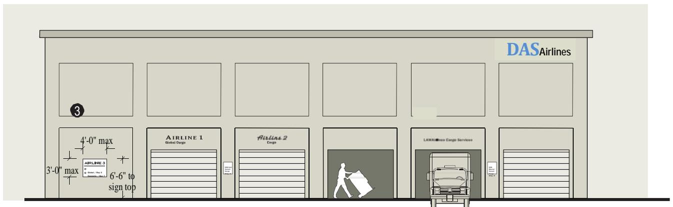
Figure 6e: Directional signs attached to tenant buildings are acceptable but not preferred.
